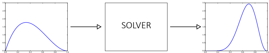
Figure: Input - airfoil thickness PDF, Output - lift force PDF
