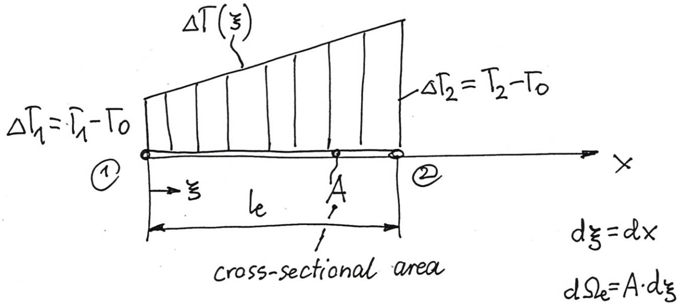
$\Delta T_1, \Delta T_2$  - nodal parameters in thermal analysis
