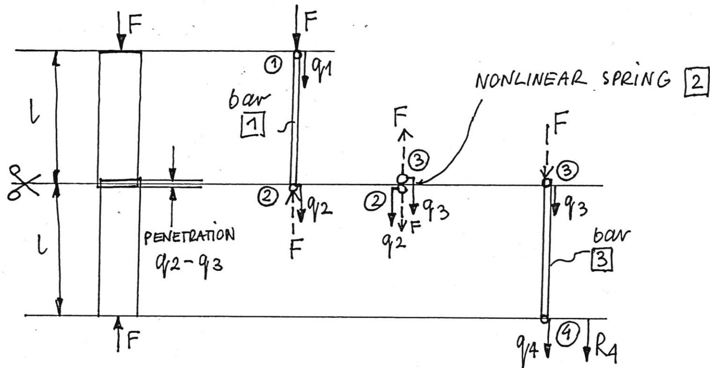
A SPRING IS ADDED TO STOP THE PENETRATION.
