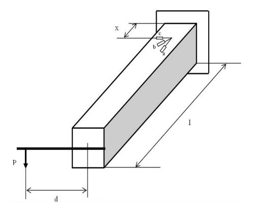
If  $d \neq 0$  the member is bent and twisted simultaneously. In order to find strain for pure torsion one has to act as follows:
