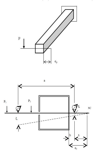
The broken line shows rotation of the cross-section around shear centre when the rod is loaded with a pair of forces  $(P_2 = -P_1)$ .  $f_a$  and  $f_b$  are displacements measured by dial indicators. These values may be found indirectly by means of the following algorithm:
