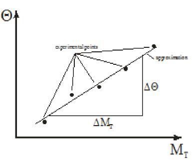
2. read  $\Delta M_T$  and  $\Delta \Theta$  from the diagram and calculate shear modulus:  $G = \frac{\Delta M_T}{\Delta \Theta} \frac{1}{J_0}$  for circular rod,  $G = \frac{\Delta M_T}{\Delta \Theta} \frac{1}{J_S}$  for rectangular rod
