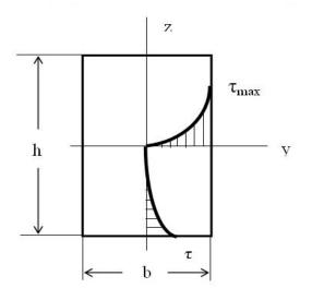
Coefficient  $k_1$  and  $k_2$  depend on b to h ratio (see table below)
