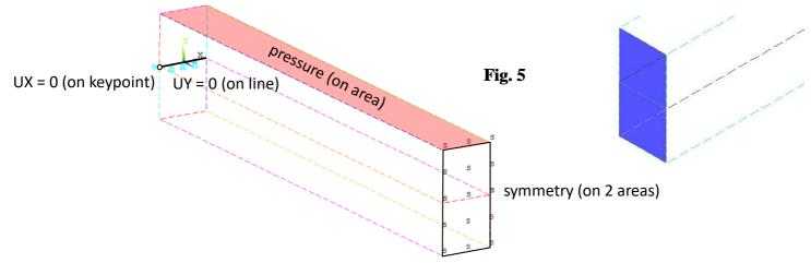
and a pressure of 10/3 MPa on the top Area(Fig. 5 and 5a) (Solution> DefineLoads>Apply> Structural> Pressure>On Areas )
